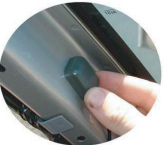
**3** Once pulled back you will see the bare metal of the "A" pillar. The GPS antenna is magnetic and will stick to pillar.
