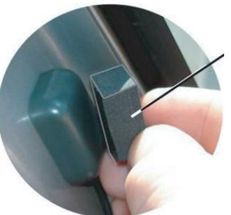
**4** Make sure the GPS is in the center of the pillar and about 3/4 the way up the pillar (from where the dash meets the windshield).
