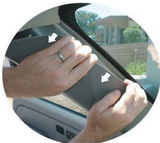
**1** The GPS antenna will have a clear view of the sky if mounted on the drivers side "A" pillar frame.
