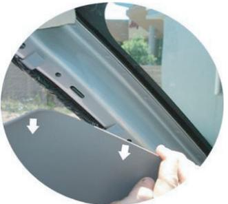
**2** To install the GPS antenna, remove the "A" Pillar cover. Start at top and carefully pull it away just slightly. It is usually held in place by clips spaced 4" apart.
